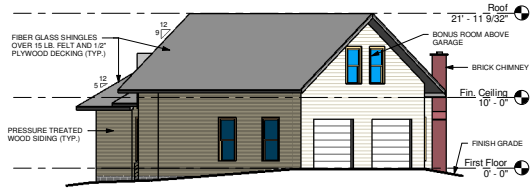
Right (East) Exterior Elevation
